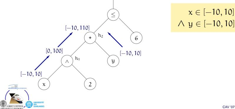
Complex constraints are rewritten to "triplets" (primitive constraints):
