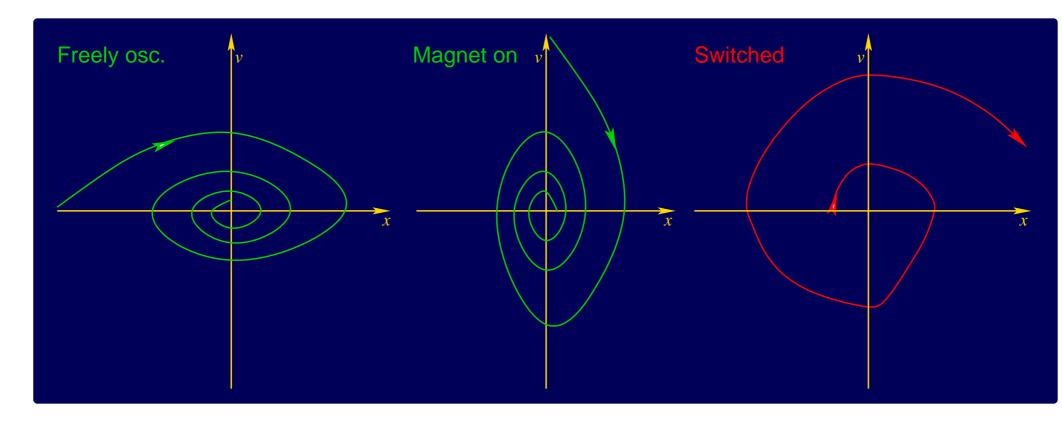
Interaction of continuous dynamics and discrete mode switch destroys global convergence!
