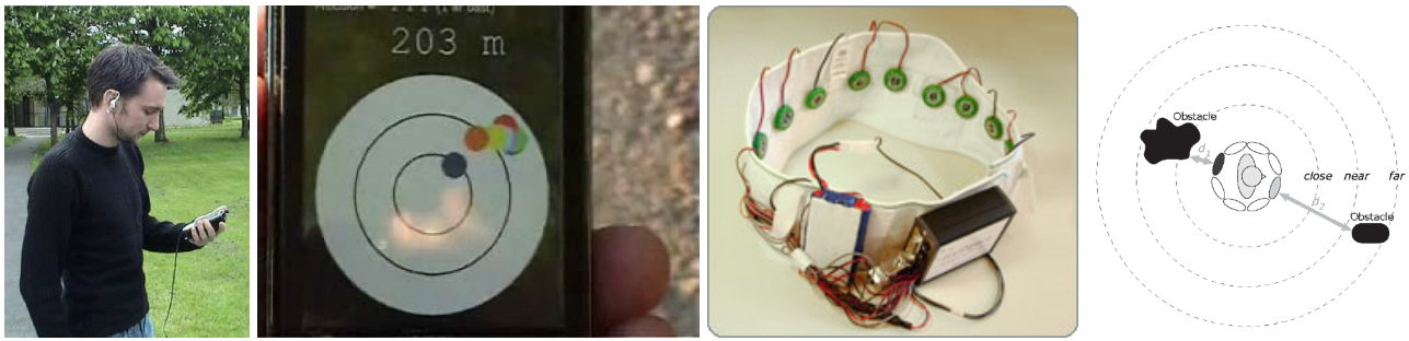
Figure 2: (a) GPSTunes [13], an auditory compass (b) SoundCrumbs [7], auditory landmark visualisation, (c) FeelSpace [8], a tactile compass, (d) Space Awareness [4] by presenting the location of obstacles by a tactile display.
