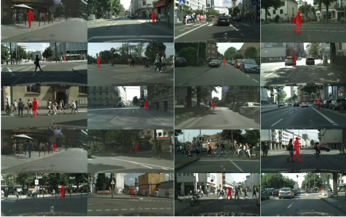
Figure 5.7: Top-5 nearest latent representations of pedestrian centers (rows) for four trained prototypes (columns).
