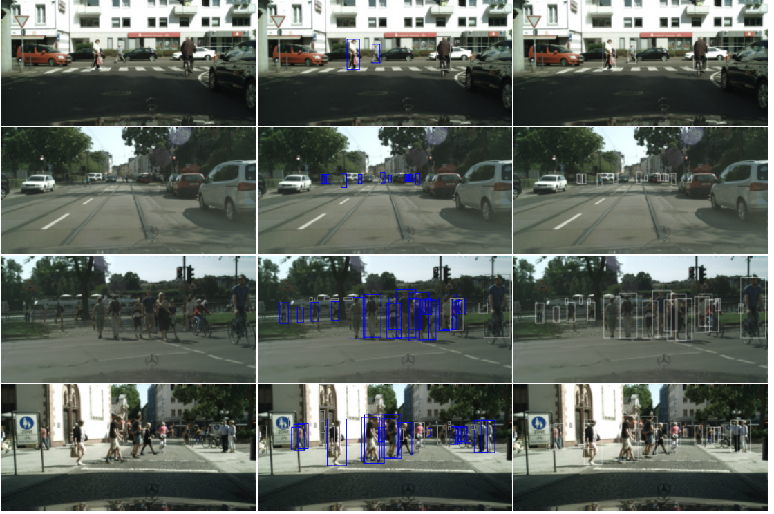
Figure 5.2: Inference results, including detection bounding boxes (white) for the DNN for center, scale and offset prediction (CSO, right column). The left column shows the original images from Cityscapes and the middle column adds the ground truth bounding boxes (blue). Gray bounding boxes are ignored. The inference is conducted with a confidence threshold of 0.4.
