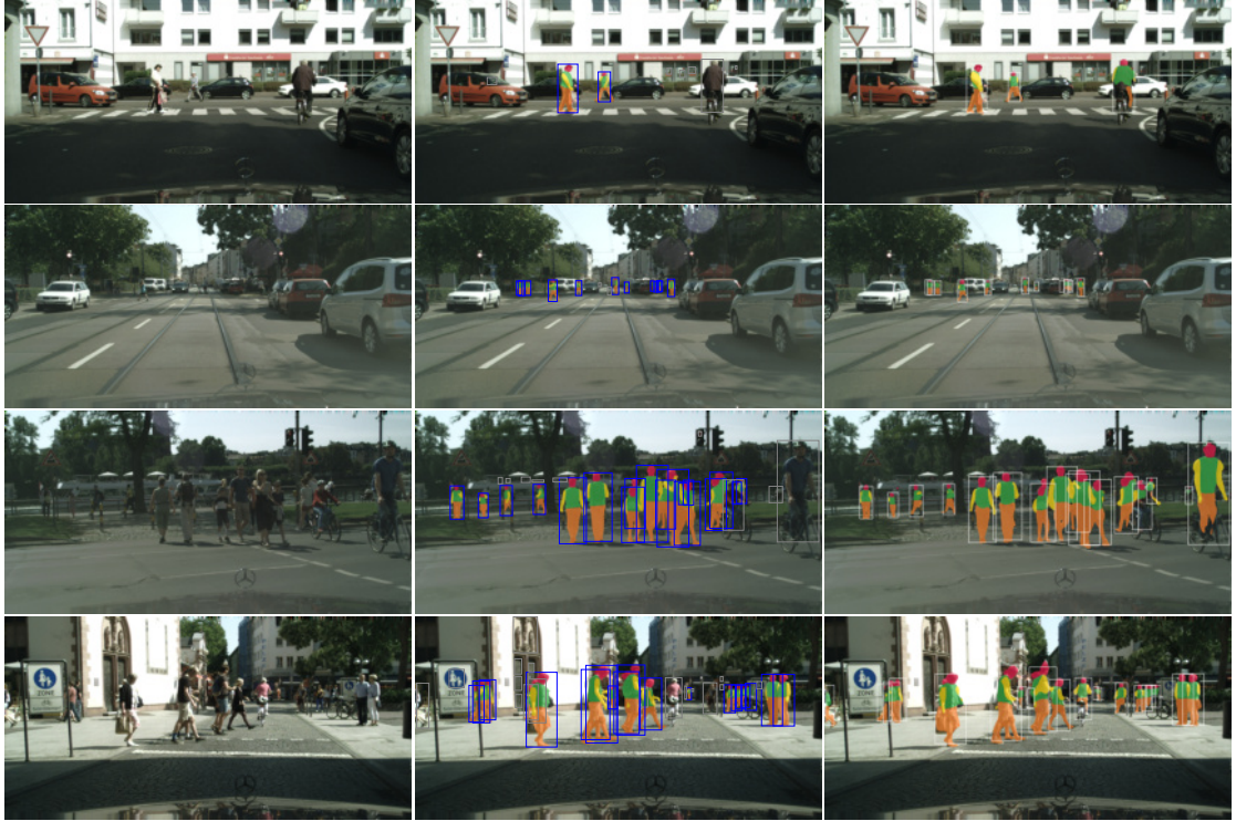
Figure 5.3: Inference results, including detection bounding boxes (white) for the DNN for center, scale and offset prediction and body part segmentation (CSOS, right column). The left column shows the original images from Cityscapes and the middle column adds the ground truth bounding boxes (blue) and body part segmentation. Gray bounding boxes are ignored. The inference is conducted with a confidence threshold of 0.4.
