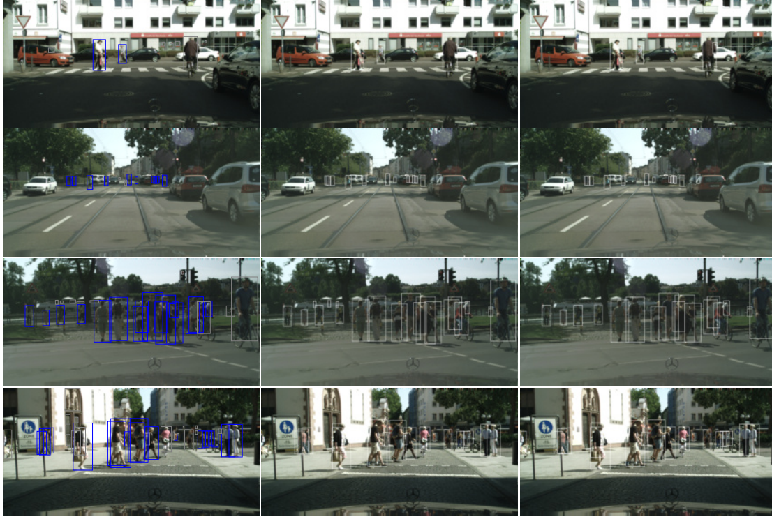
Figure 5.5: Inference results, including detection bounding boxes (white) for the DNN for prototype-pedestrian detection (PPD, right column) and the DNN for center, scale and offset prediction (CSO, middle column). The left column shows the original images from Cityscapes with ground truth bounding boxes (blue) and ignored bounding boxes (red). The inference is conducted with a confidence threshold of 0.4.
