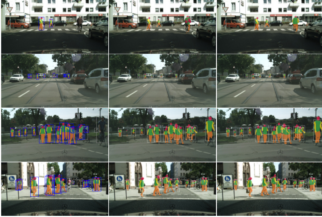
Figure 5.13: Inference results, including detection bounding boxes (white) for the DNN for concept-based domain adaptation for pedestrian detection (ConDA, right column) and the DNN for concept-based pedestrian detection (CPD, middle column). The left column shows the original images from Cityscapes with ground truth bounding boxes (blue) and the body part segmentation. The inference is conducted with a confidence threshold of 0.4.
