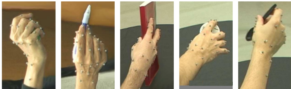
Figure 2.3: Examples of Hand motion tracking using optical markers in object manipulation tasks [CPMX07].
