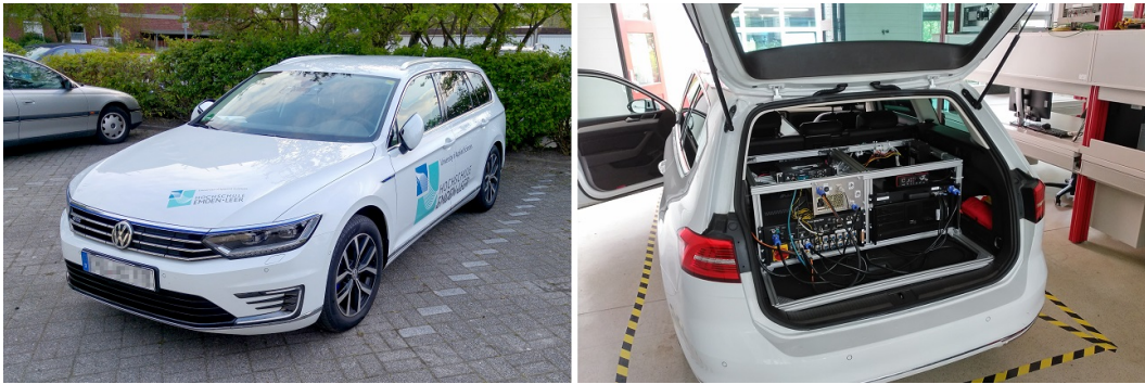
Figure 6.21: The measurement vehicle used within the FASva project with the measurement system located in the trunk of the vehicle (right panel). © Hochschule Emden/Leer
