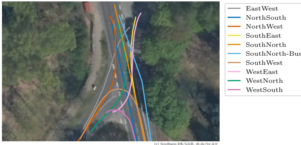
Figure 6.19: An example application of TASI for route estimation without a digital representation of the road network. The reference line for each routing direction is estimated based on trajectories from a subset of the overall data set.
