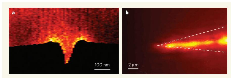
**Figure 2 | Into the groove.** **a**, Ropers and colleagues' 'tip-enhanced electron emission microscopy'<sup>1</sup> provides a picture of a nanoscale groove in a gold surface. **b**, The laser-illuminated probe tip.
