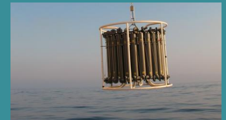
So-called rosette samplers are used to take water samples at different water depths. [Foto: Nelli Sergeeva]
