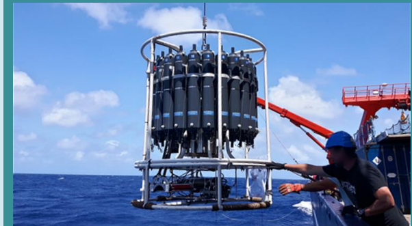
Water samples collected in the North Atlantic Ocean by deploying a rosette, containing Niskin bottles and physical sensors [Photo: M. Seidel]
