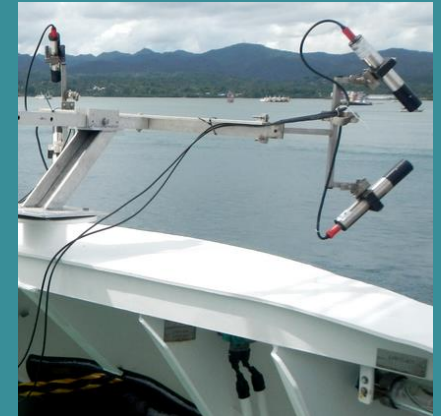
Bow of the research vessel SONNE with installed radiometer [© ICBM/ Shungudzemwoyo P. Garaba]
