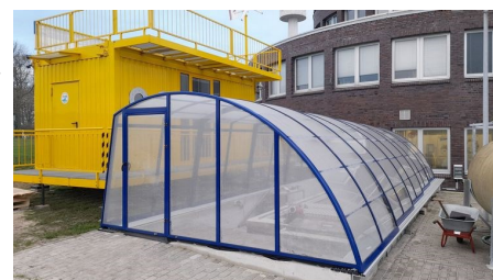
The yellow display container is the future control centre for real-time measurements in the ICBM's covered outdoor basin [Photo: H. Nicolai, ICBM]
