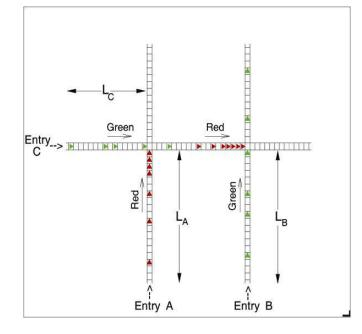
Efficiency of green-wave method strongly depend on The traffic volumes in the Perpendicular streets.
