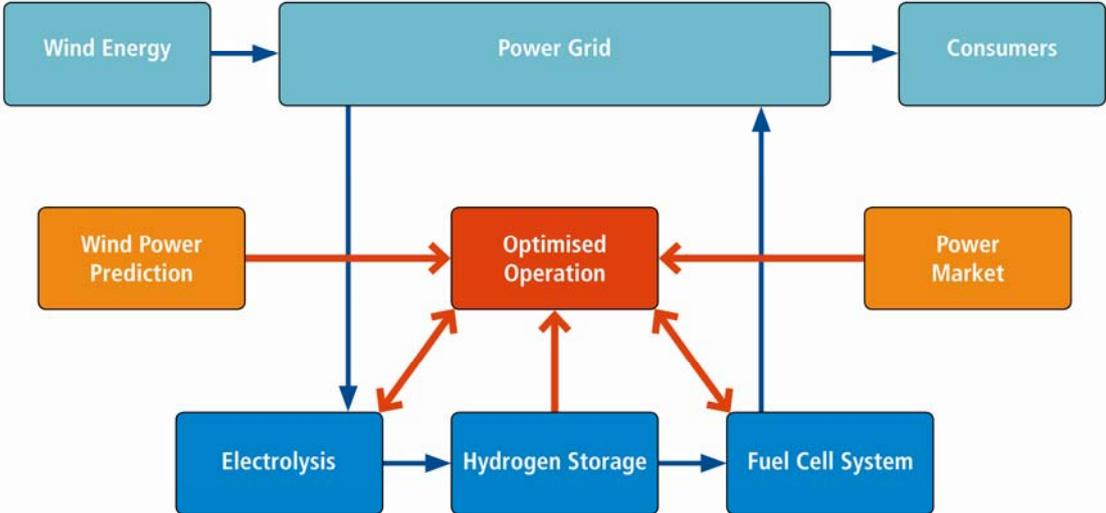
Figure 1: Principal structure of the *HyWindBalance* wind-hydrogen storage system.
