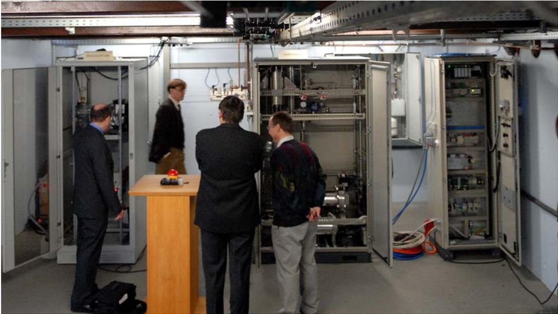
Figure 2: View of the laboratory setup of the *HyWindBalance* experimental system during the official inauguration. From left to right: fuel cell unit, electrolyser, electrical control unit.
