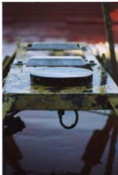
Figure 9: Sensor of the acoustic wave recorder
