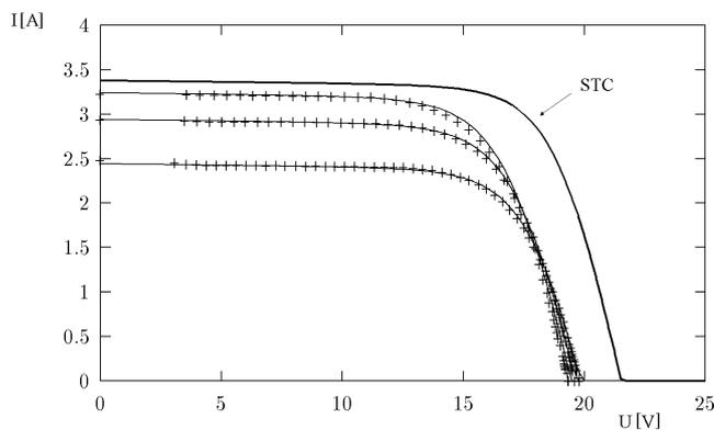
Fig. 2.1. Measured I-V characteristic (+), results of the parameter fit for the two diode model (-) and the calculated I-V characteristic under STC derived from the parameter fits.
