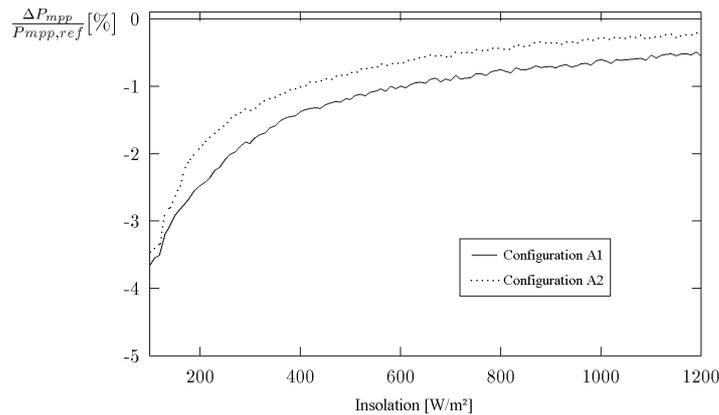
Fig. 3.6. Power losses in a 5.3 kW<sub>p</sub> PV array for different irradiance values. The module temperature is assumed to be constant 25 °C.
