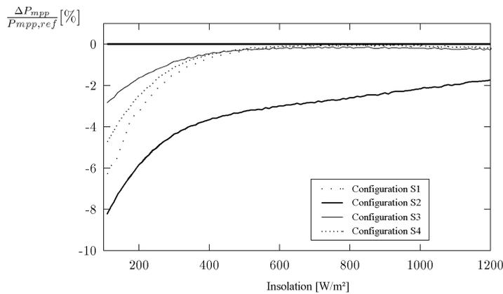
Fig. 3.2. Relative power loss depending on the irradiance for the various string configurations exemplary for a module temperature of 25 °C. The reference is a PV string consisting of 20 modules with identical I-V characteristics.
