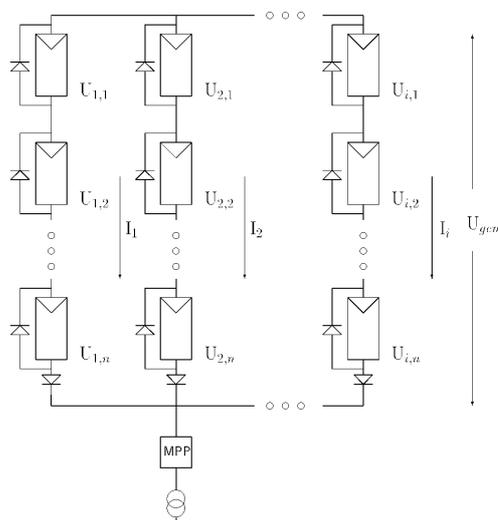
Fig. 3.4. PV array used for the calculations.
