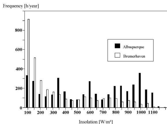
Fig. 3.3. Frequency distribution of hourly irradiation values for the data sets used.
