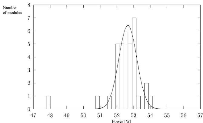
Fig. 2.2 MPP power distribution of the 36 individual modules under Standard Test Conditions.
