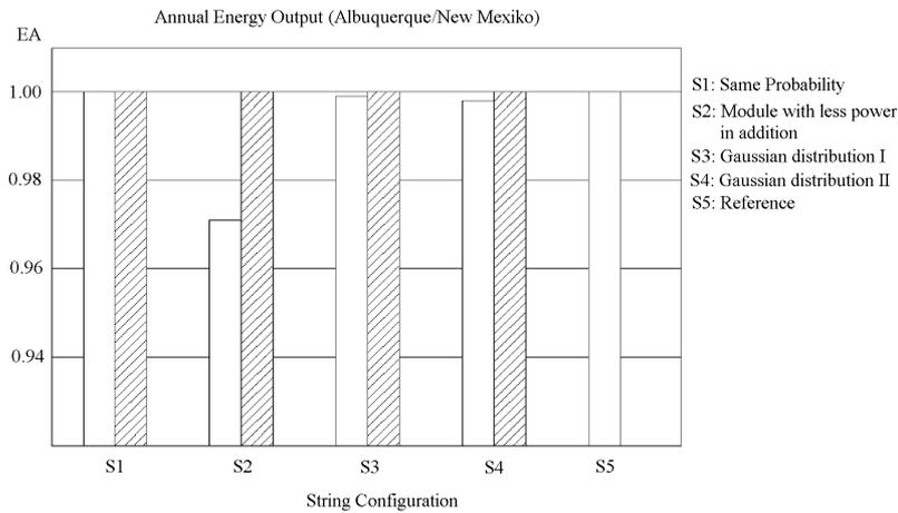
Fig. 3.1 Results of the calculations of the mismatch losses for different string configurations. The reference string consists of 20 modules with identical I-V characteristics.
