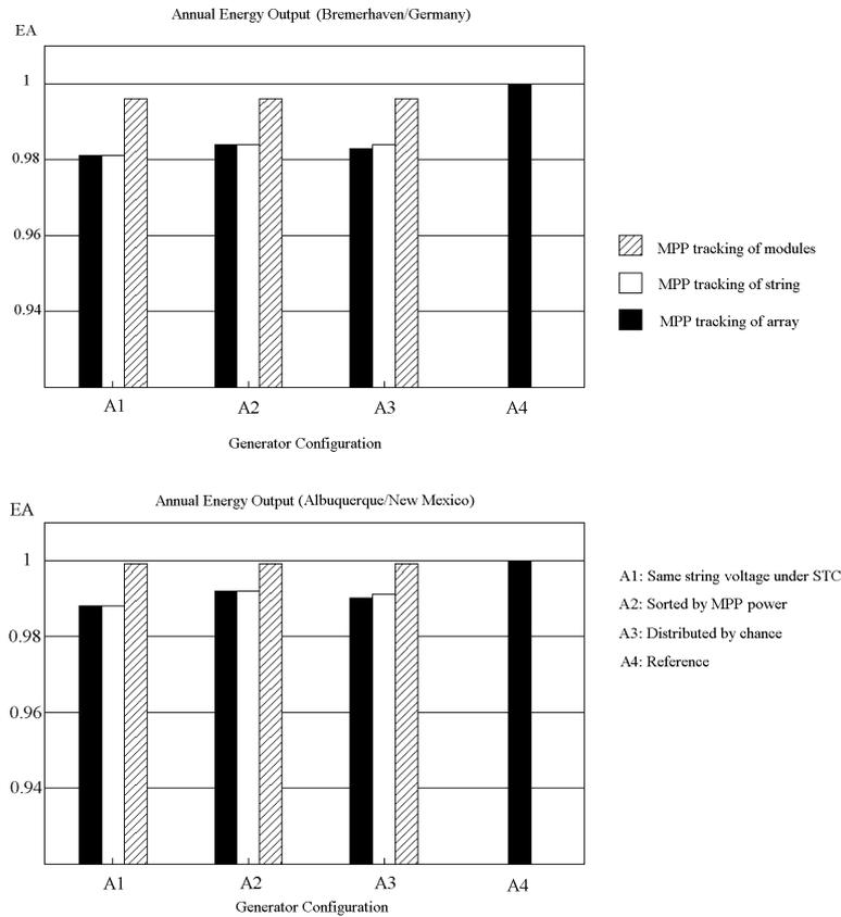
Fig. 3.5. Results of the calculations of the mismatch losses for different generator configurations. The reference generator consists of 100 modules with identical I-V characteristics.
