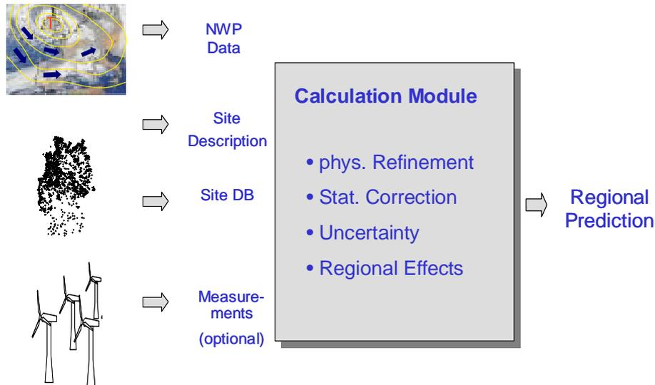
Figure 4: Principle function of the prediction system Previento
