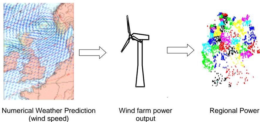
Figure 1: Principle of wind power prediction from the numerical weather prediction to the regional wind power.
