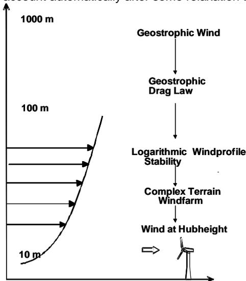
Figure 2: Local refinement of the numerical prediction with physical models
