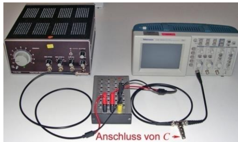
Fig. 13: Picture of the circuit from Fig. showing the function generator on the left, the oscilloscope on the right, and the resistance decade with resistor R_D in the centre. R_D is located between the two black terminals of the resistance decade. The yellow terminal is a support contact without an electrical connection to R_D . A BNC-T connector is inserted in the cable connecting the resistance decade and the oscilloscope in order to connect the capacitor for which the capacitance C is to be determined.
