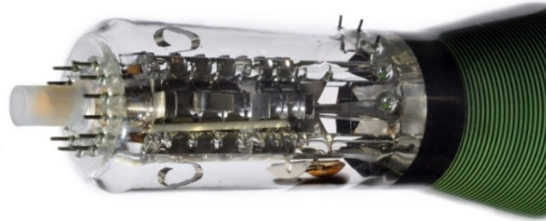
Fig. 2: Photograph of the back-end of an cathode ray oscilloscope tube. It shows the complex structure of the electrodes for forming and controlling the electron beam. The connecting contacts for the different electrodes can be seen at the end of the tube and on the right side of the casing.
