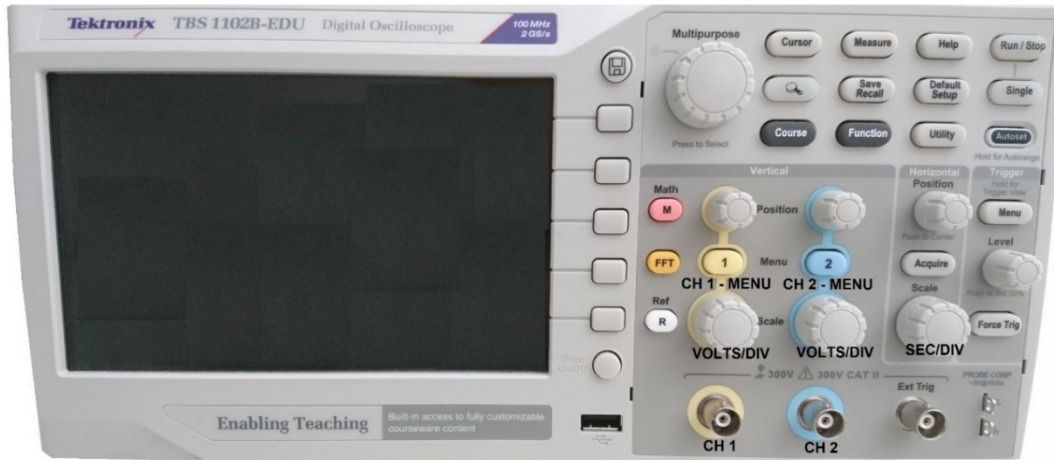
Fig. 9: Front view of the digital oscilloscope TEKTRONIX TBS 1102B EDU.
