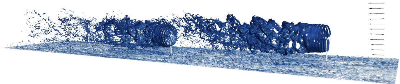
Visualization of the flow field of two interacting wind turbines by means of vorticity iso-surfaces. Results obtained from LBM-LES using an actuator line wind turbine model.
