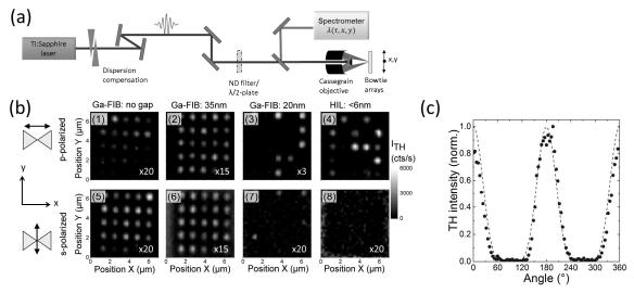
Figure 4 (a): Experimental set-up of the ultrafast nonlinear microscope. Dispersion-balanced, 8-fs laser pulses from a Ti:Sapphire oscillator are focused onto the plasmonic antenna structures using an all-reflective Cassegrain objective. Nonlinear emission from the sample is collected in reflection geometry, dispersed in a spectrometer and detected with a CCD camera.
