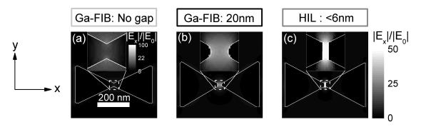
Figure 5 (a): Finite element method calculations of the electric near field enhancement  $|E_x|/|E_0|$  after excitation with optical pulse polarized along the x-direction. The pulse spectra match those used in experiment. (a) Ga-FIB antenna without gap, (b) Ga-FIB antenna with a gap of 20nm and (c) a He-FIB antenna with a gap of less than 6 nm. The insets in the Figures show a zoom into the gap region of the antenna with a two times larger enhancement scale.
