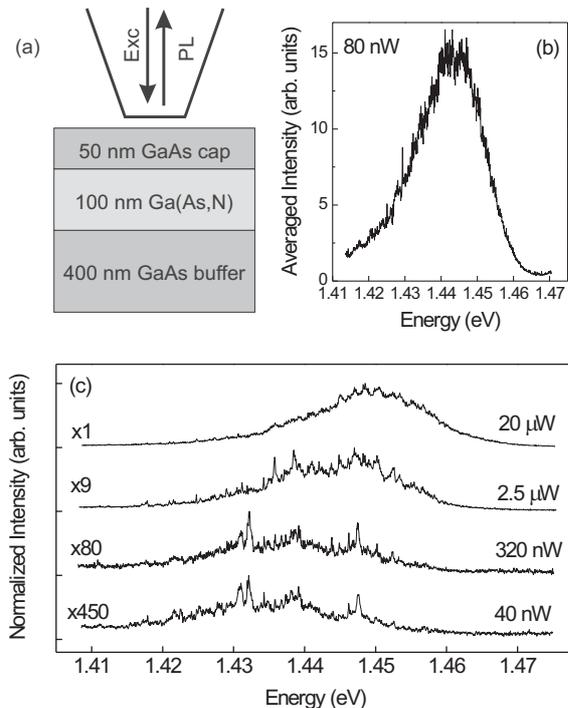
FIG. 1: (a) Schematic of the experimental setup. (b) Spatially averaged PL spectrum of the  $\text{GaAs}_{0.999}\text{N}_{0.001}$  sample at  $T = 10$  K, taken from 1600 NSOM spectra. (c) Individual near-field PL spectra recorded for different excitation powers at the same spot of the sample.
