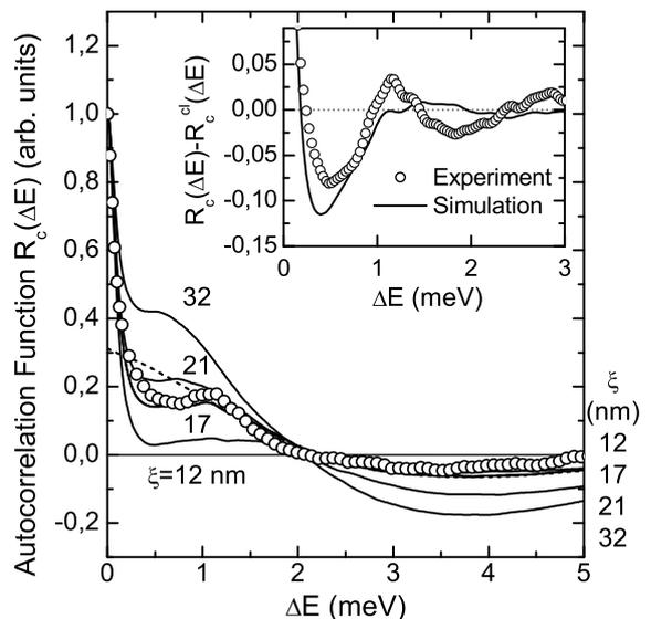
FIG. 2: Experimental (circles) and simulated (solid line) autocorrelation functions  $R_c(\Delta E)$ . The simulations were performed for a disorder amplitude of  $2.1\text{ meV}$  and correlation lengths  $\xi$  of  $12\text{--}32\text{ nm}$ . Dashed line: Classical limit ( $M \rightarrow \infty$ ) for  $\xi = 17\text{ nm}$ . Inset: Deviation between experimental (circles) and simulated (line) data and the classical limit.
