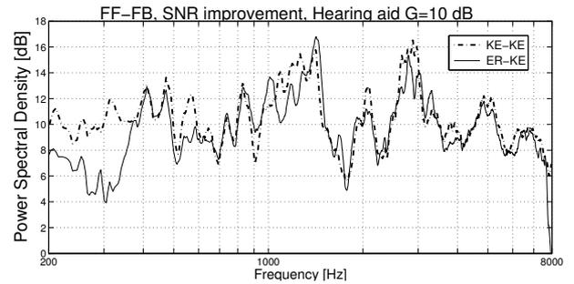
Figure 6: Frequency-dependent SNR improvement  $\Delta SNR_j$  of the combined FF-FB ANC motivated algorithm, at the KEMAR microphone (cases KE-KE and ER-KE,  $G = 10$  dB).
