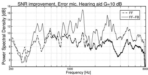
Figure 4: Frequency-dependent SNR improvement  $\Delta SNR_j$  of the ANC motivated algorithms at the error microphone (case ER-ER,  $G = 10$  dB).
