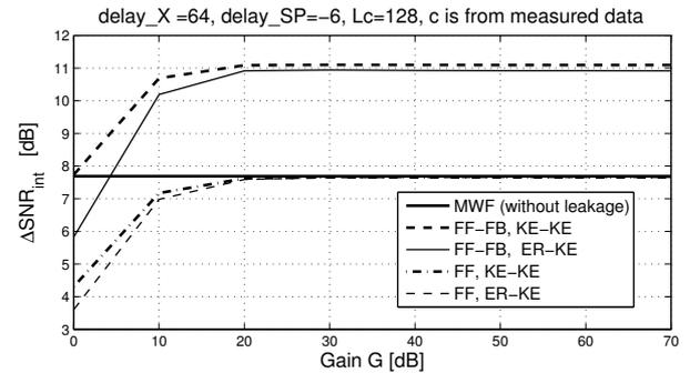
Figure 5: Speech intelligibility-weighted SNR improvement  $\Delta SNR_{int}$  of the FF ANC and the combined FF-FB ANC motivated algorithms at the KEMAR microphone (cases KE-KE and ER-KE).
