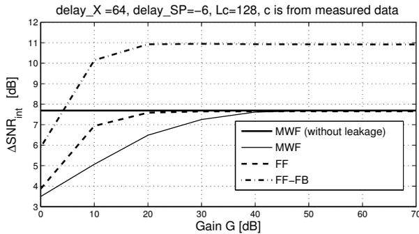
Figure 3: Speech intelligibility-weighted SNR improvement  $\Delta SNR_{int}$  of the MWF (with/without leakage) and ANC motivated algorithms at the error microphone (case ER-ER).
