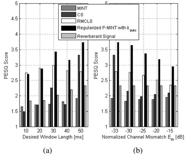
Fig. 6. PESQ score of the first microphone signal  $x_1(n)$  and PESQ score of the system's output  $\hat{s}(n)$  obtained using MINT, CS, RMCLS, and regularized P-MINT with  $\delta_{\text{auto}}$  for (a) several desired window lengths ( $E_m = -33$  dB) and (b) several normalized channel mismatches ( $L_d = 50$  ms)
