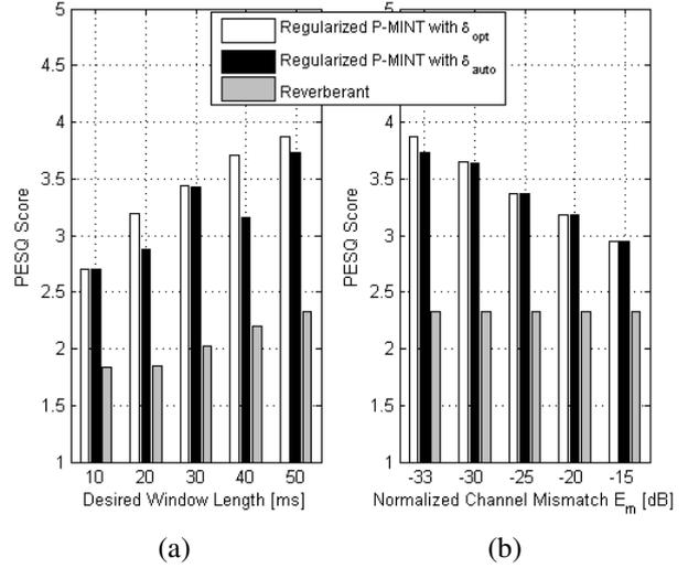
Fig. 4. PESQ score of the first microphone signal  $x_1(n)$  and PESQ score of the system's output  $\hat{s}(n)$  obtained using regularized P-MINT with  $\delta_{\text{opt}}$  and  $\delta_{\text{auto}}$  for (a) several desired window lengths ( $E_m = -33$  dB) and (b) several normalized channel mismatches ( $L_s = 50$  ms)
