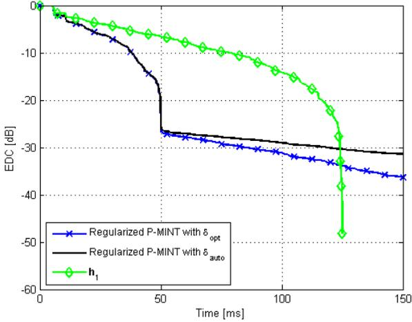
Fig. 3. EDC of the true RIR  $\mathbf{h}_1$  and EDC of the EIR using regularized P-MINT with  $\delta_{\text{opt}}$  and  $\delta_{\text{auto}}$  ( $E_m = -33$  dB,  $L_s = 50$  ms)
