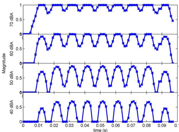
**Fig. 3.** Illustration of reduced modulation depth with increasing input sound pressure level. The input signal was a speech weighted click train with an F0 of 100 Hz, at different input levels. The pulses on the fourth most apical electrode are shown. Magnitudes between 0 and 1 are mapped to current units between threshold and comfortable loudness.
