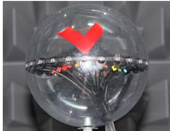
FIGURE 5: VAH with 24 equidistantly spaced microphones (Sennheiser KE-4) on the horizontal plane. The microphones are mounted flush in a rigid sphere with a diameter of \approx 18 cm.
