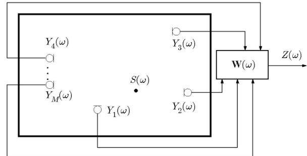
Fig. 1. Configuration of a sensor network with  $M$  microphones.
