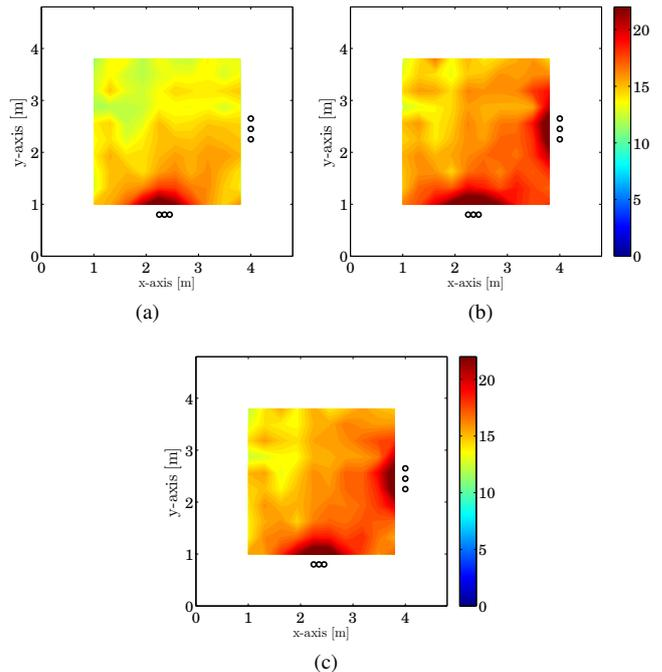
**Fig. 4.** Position-dependent broadband output SNR of the different MWF filters: (a) S-MWF; (b) R1-MWF; (c) A-MWF.
