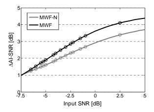
**Fig. 1:**  $\Delta$ AI-SNR for MWF (black) and MWF-N (grey) as a function of input SNR. Circles denote individual test SNRs.
