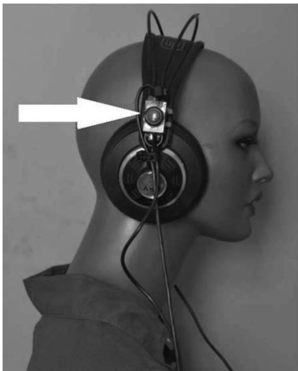
Fig. 6. Headphones. Headphones seated on the DH 2 with a toggle button (cf., white arrow) that allows to switch between the test and the reference setting.
