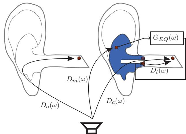
**Figure 1:** Considered acoustic scenario with acoustic transfer functions and signal processing blocks.
