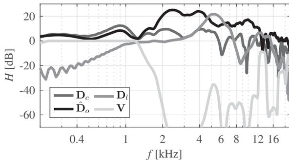
**Figure 2:** Acoustic transfer functions utilized for the simulations. The regularization weight  $\mathbf{V}$  was calculated according to Eq. (17)
