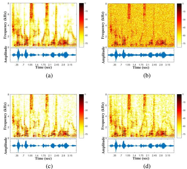
Fig. 3. Spectrograms of (a) clean signal, (b) noisy signal, (c) enhanced signal using MCMF-MVDR filter, and (d) the enhanced signal using proposed SDMCMF-MVDR filter (SNR =  $10 \text{ dB}$ , white Gaussian noise).
