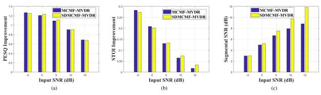
Fig. 4. Performance of the proposed SDMCMF-MVDR and MCMF-MVDR in terms of PESQ, STOI and SSNR in the case of factory noise
