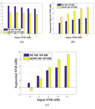
Fig. 2. Performance of the proposed SDMCMF-MVDR and the MCMF-MVDR filters in terms of SegNR, SSPSNR and SSNR for several SNRs (white Gaussian noise)
