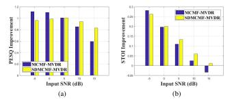
Fig. 1. Performance of the proposed SDMCMF-MVDR and the MCMF-MVDR filters in terms of PESQ and STOI improvement compared to the noisy signal for several SNRs (white Gaussian noise)
