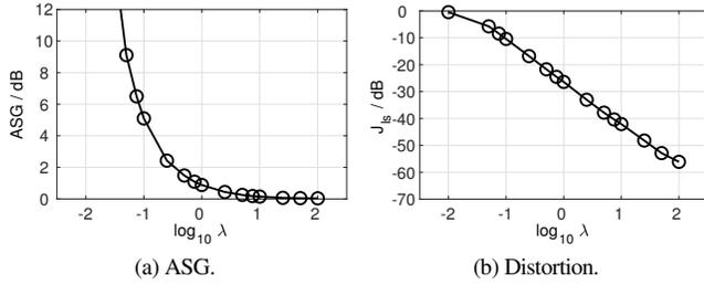
Figure 3: Added stable gain and distortion for the optimal performance in Experiment 1.
