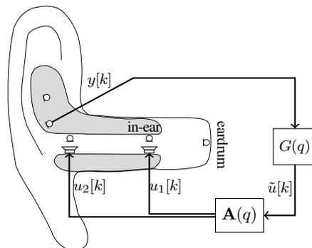
Figure 1: Schematic overview of considered single-microphone multi-loudspeaker hearing device setup.
