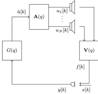
Figure 2: Considered multi-loudspeaker single-microphone hearing device setup.
