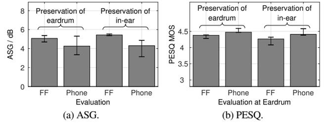
Figure 4: Evaluation results of Experiment 2 in terms of (a) the median ASG and (b) the median PESQ MOSs. Errorbars show minimum and maximum values, respectively. Results are shown for both conditions when the acoustic path between the loudspeakers and the eardrum is known (preservation of eardrum) and when the acoustic path between the loudspeaker and the eardrum is estimated using an in-ear microphone (preservation of in-ear).
