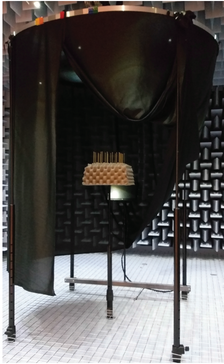
Figure 2: The VAH inside the acoustically transparent curtain at Listener Position. During the both listening tests subjects were seated at the Listener Position inside this curtain.
