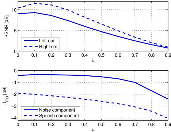
Figure 2: SNR improvement and ITD cost function using partial estimation of the noise component ( $M = 4$ ,  $\text{SNR}_0 = 0$  dB,  $\beta = 0$ )
