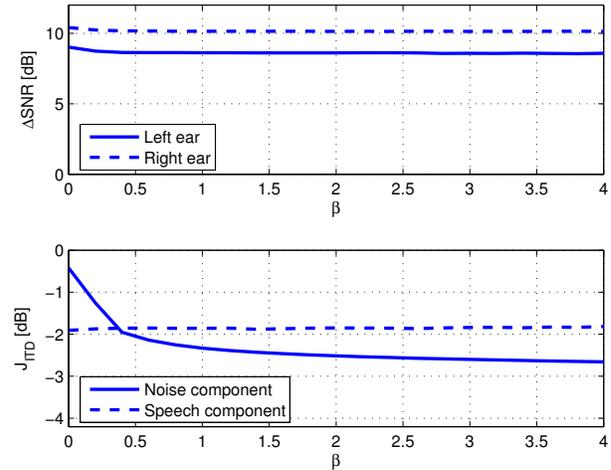
Figure 3: SNR improvement and ITD cost function using extension of MWF with ITD cues ( $M = 4$ ,  $\text{SNR}_0 = 0$  dB,  $\lambda_0 = \lambda_1 = 0$ )
