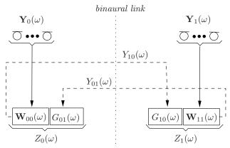
Figure 2: Distributed binaural MWF scheme (dB-MWF)
