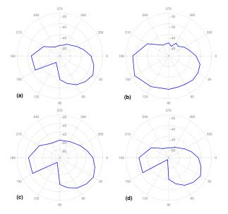
Figure 6: Spatial directivity pattern of  $\mathbf{F}_{01}$  with  $\theta_v = 120^\circ$  for (a) B-MWF, (b) MWF-front, (c) MWF-contra, (d) dB-MWF
