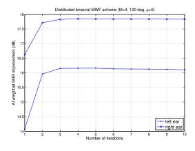
Figure 5: SNR improvement at left and right hearing aid with  $\theta_v = 120^{\circ}$  for dB-MWF as a function of the number of iterations
