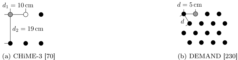
Figure 7.2: Considered microphone array geometries. Grey circles denote the reference microphone and white circles denote unused microphones.
