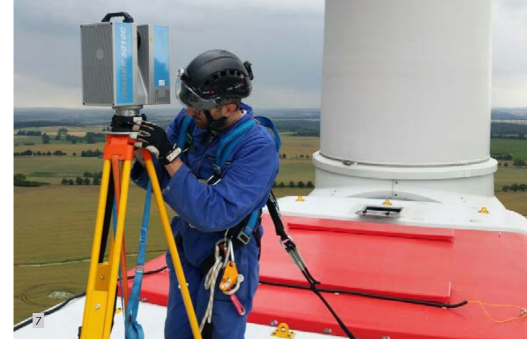
7 At open area test sites the scientists measure the "real" external influences to which the wind farm is exposed. The photo shows a 3D scanner being set up.
