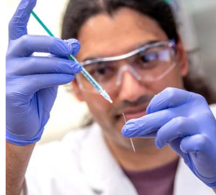
To close the circuit with the negatively polarized cathode, Karuna Kanes positions a hair-thin wire – the anode – inside the printing nozzle.
