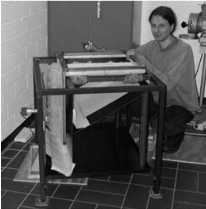
Figure 3.23. The shaking machine used to measure attachment capacity. A comb is used to homogenise the coat and to comb the seeds into the wool or hair.
