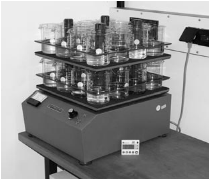
Figure 3.22. Measurement of the floating capacity of seeds using a flaskshaker.
