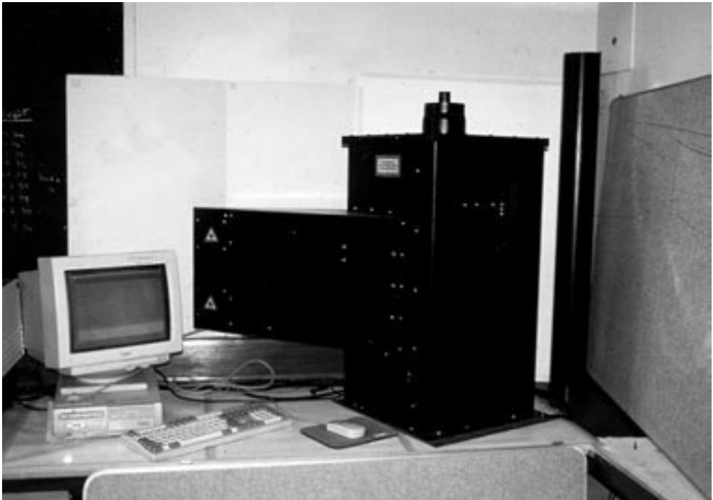
Figure 3.21. Experimental set up for the measurement of the terminal velocity of dispersal units.
