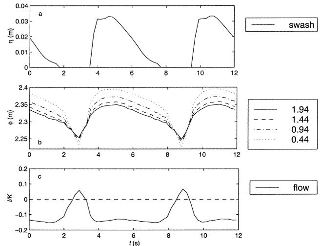
Fig. 14. (a) Simulated swash depth at  $x = 23.9$  m over two wave periods. (b) Head variations at different depths (i.e.,  $z_b z$ ; the values are listed in the legend box). (c) Time-varying rates of local infiltration/exfiltration.
