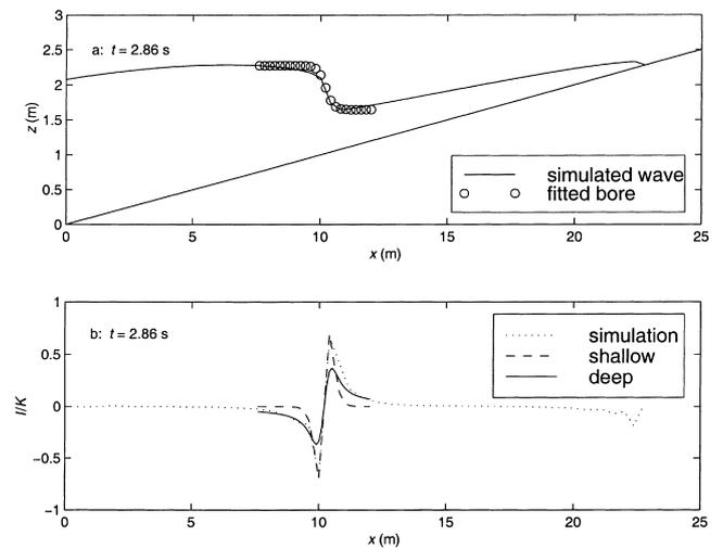
Fig. 5. Comparison of the simulated bore (a) and infiltration/exfiltration (b) with analytical solutions by Packwood and Peregrine [11] for  $t = 2.86$  s.
