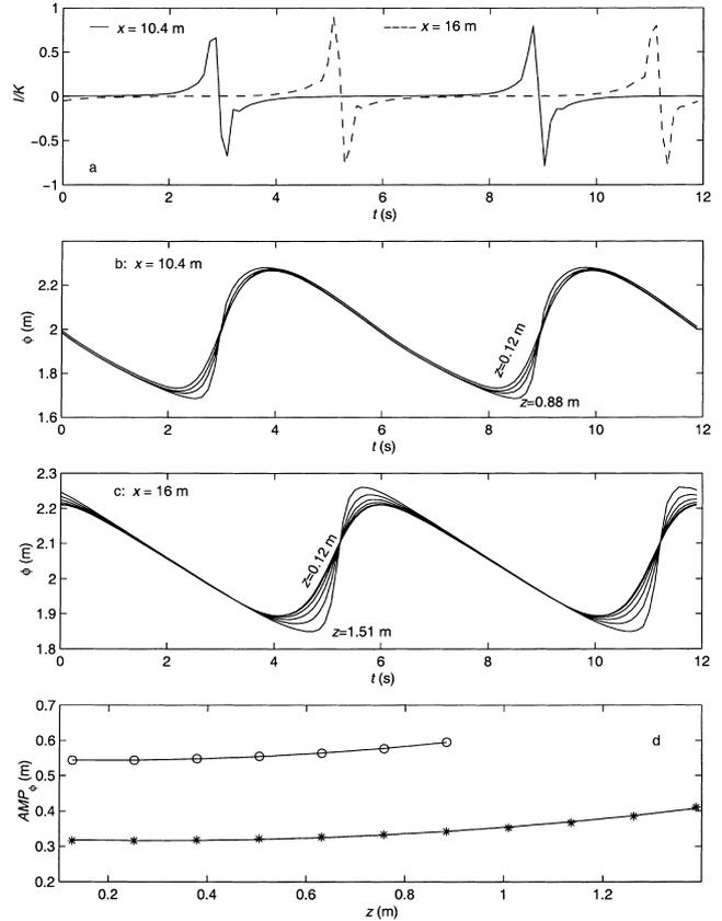
Fig. 12. (a) Time-variations of infiltration/exfiltration at fixed locations. (b) Head fluctuations at different depths for  $x = 10.4$  m. (c) head fluctuations at different depths for  $x = 16$  m. (d) depth variations of the amplitude of head fluctuations at  $x = 10.4$  m (circles) and  $x = 16$  m (stars).
