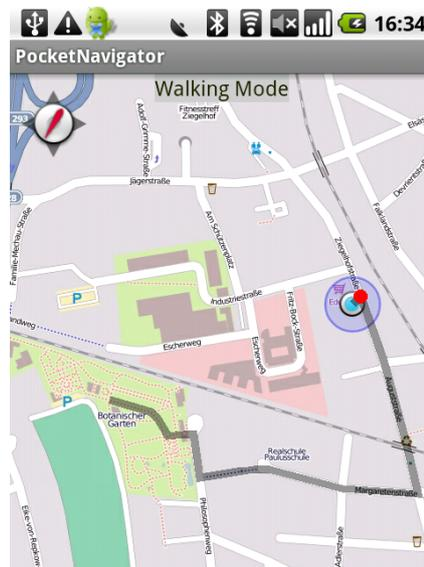
**Figure 2: A screenshot of the PocketNavigator's main view: similarly to many map-based navigation systems the user's position is shown on a map (here OpenStreetMap.org) and optionally the current route is highlighted.**
