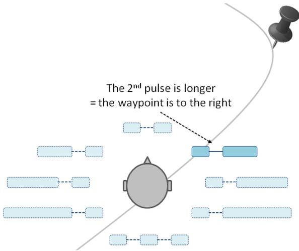
**Figure 3:** Instead of giving turning instructions, such as "turn left now", the PocketNavigator uses a Tactile Compass to point towards the current waypoint. By walking into the pointing direction the user is guided from one waypoint to another until reaching the destination.
