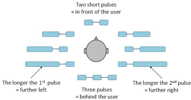
**Figure 4:** *TwoPulse* direction encoding: the direction in which the waypoint is encoded in the relative length of two pulses. The further left/right the waypoint is the longer the first/second pulse becomes.
