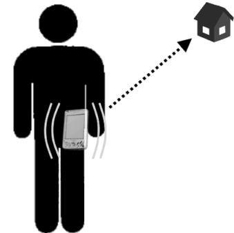
Figure 1: The basic idea: a "Tactile Compass" encodes - in vibration patterns generated by an everyday mobile phone - in which direction and how far a place is located from the perspective of the user.
