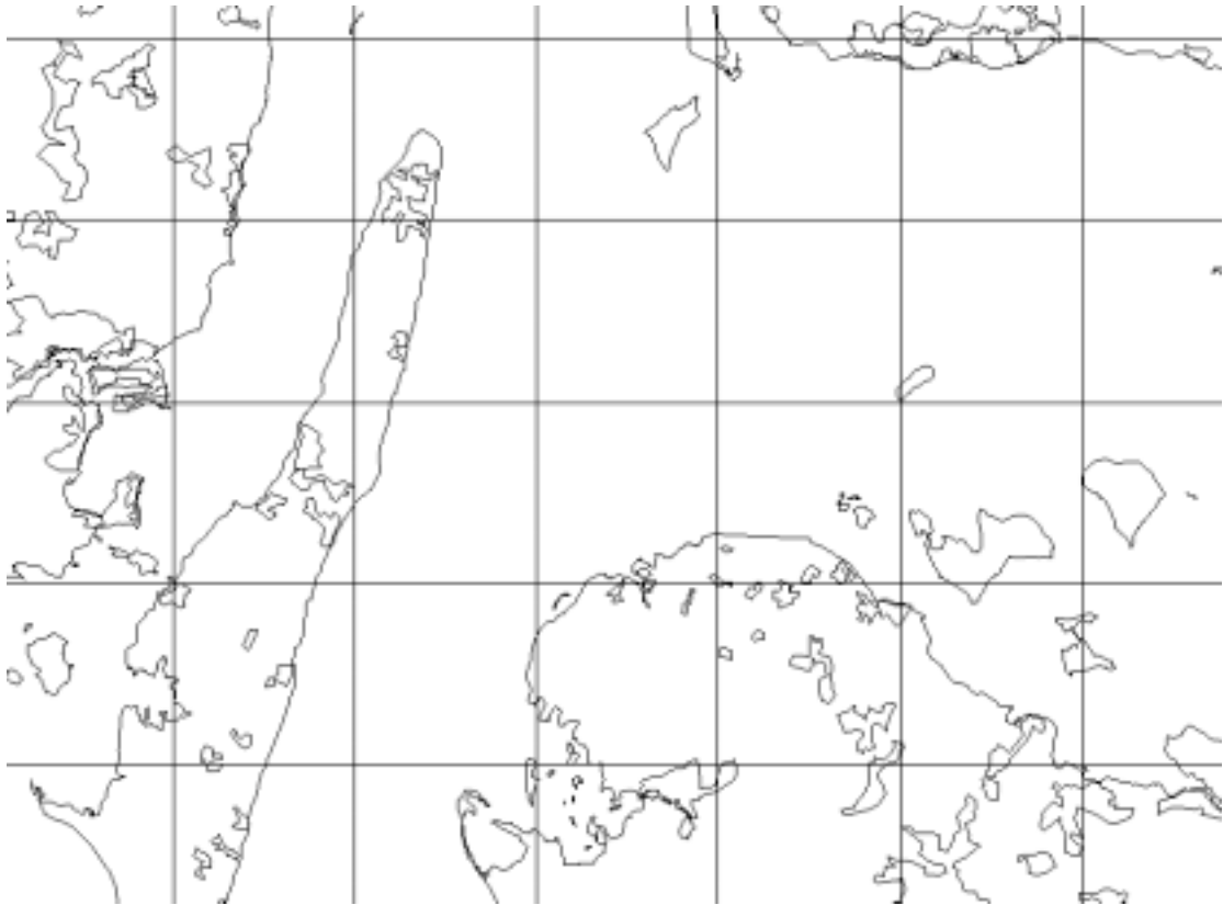
Figure 4: Map of roughness change lines around the Vindeby and Omø Stålgrunde sites; the distance between the grid lines is 10km; roughness values used: 0.0m for water, 0.05m for agricultural areas and 0,4m for cities and forests
