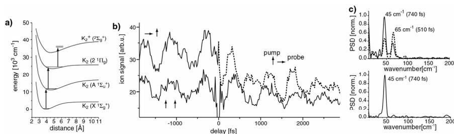
**Fig. 1.** a) Calculated potential energy curves of the potassium dimer system. b) Section of pump–probe transients with mutually parallel (solid line) and crossed (dashed line) linear polarizations around delay time zero. c) FFT-analysis of pump–probe transients with parallel (lower graph) and crossed (upper graph) mutual polarizations.
