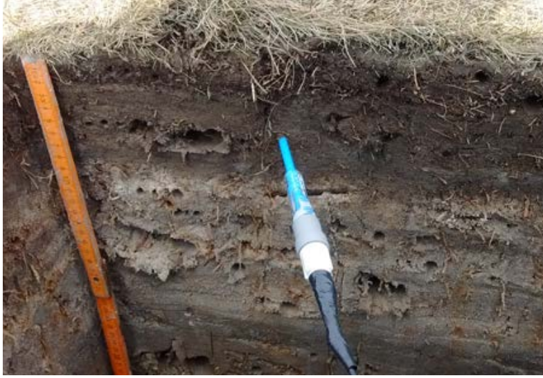
Redox potential measurements show whether aerobic or anaerobic conditions prevail in the soil.
