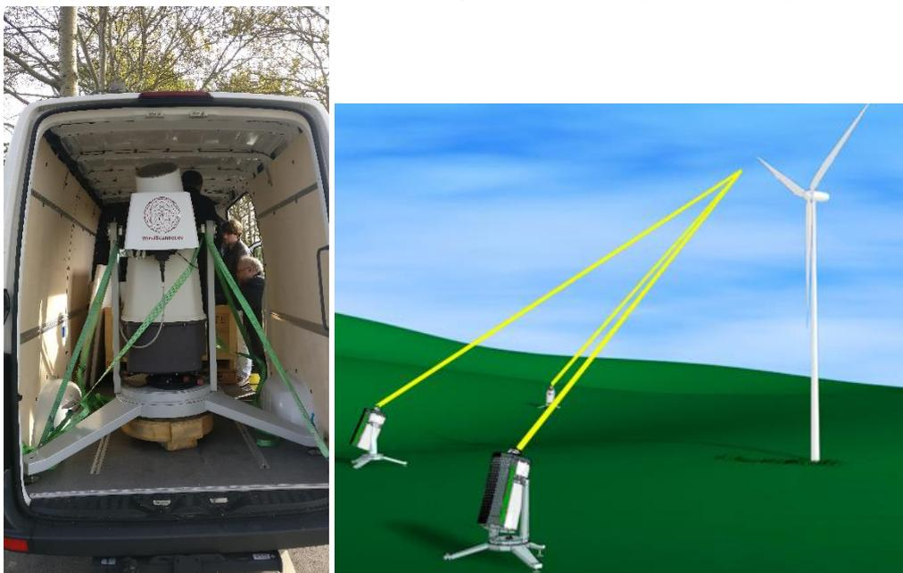
Figure 1: The 6” windscanner obtained by Uni Oldenburg and the setup of 3D wind scanners (source: DTU)
