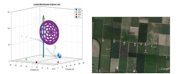
Figure 2: Locations and orientation of the lidar devices. The virtual met mast is created by the three wind scanners on the spinner lidar measurement plane.
