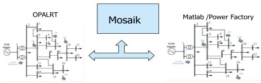
Alongside with the study part , was trying to implement a real time model validation scenario . The scenario planned was using the sensors values from a power system model simulated in the OPALRT system a digital twin of the same is created and run as a power factory/matlab simulation in real-time using the mosaik framework.
