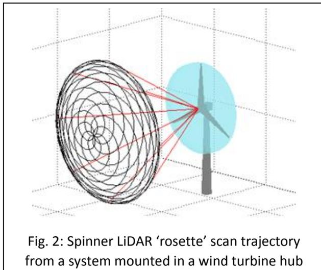
Fig. 2: Spinner LiDAR 'rosette' scan trajectory from a system mounted in a wind turbine hub
