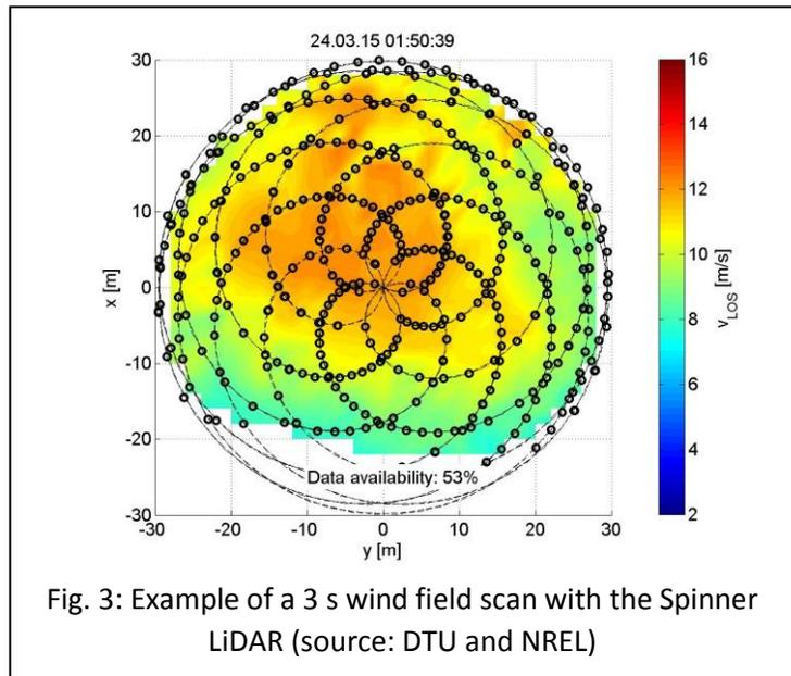
Fig. 3: Example of a 3 s wind field scan with the Spinner LiDAR (source: DTU and NREL)
