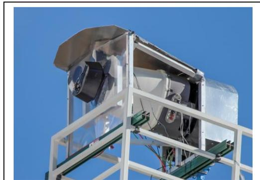
Fig. 1: Spinner LiDAR mounted on the nacelle of the CART 3 turbine at NREL, Colorado (source: DTU and NREL)
