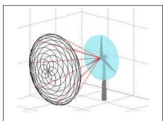
Fig. 2: Spinner LiDAR 'rosette' scan trajectory from a system mounted in a wind turbine hub
