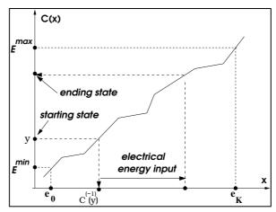
**Figure 1** This is a piecewise-constant charging illustration of the storage dynamics (for discharging similar).  $E^{min}$  and  $E^{max}$  describe the allowed energy levels of the storage. y is the state of charge, C is related to the charging rate depending on y the state of charge of the storage.
