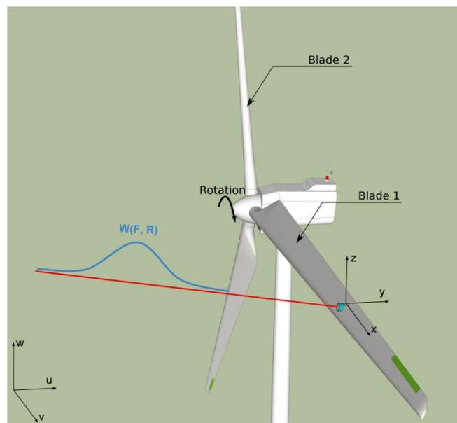
Figure 1: LiDAR measurement configuration, where a telescope is mounted on each blade and is connected through fiber optics to a continuous-wave LiDAR placed in the hub. The LiDAR is sampling the inflow wind speed in front of the wind turbine blade at a sample rate of 50 Hz, and the measurements are used to control the next blade's flap and pitch angle.
